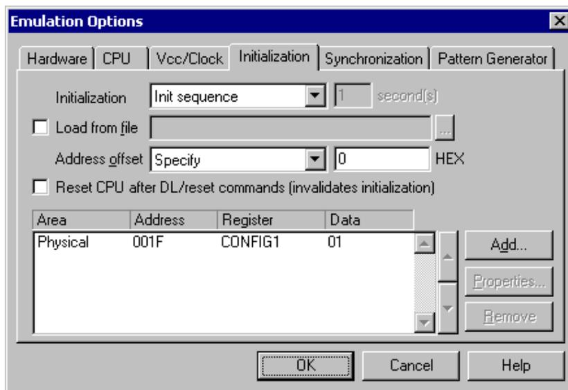
2. winIDEA accepts initialization sequence as a text file with .ini extension. The file must be written according to the syntax specified in the appendix in the hardware user's guide.
