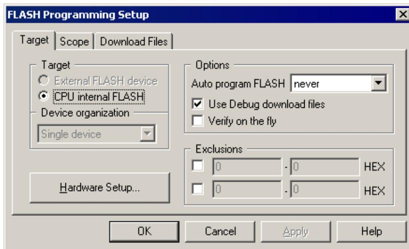
When the CPU internal flash is programmed, winIDEA takes care of most of the necessary settings. Don't check 'Verify on the fly' option since this functionality cannot be supported on this CPU family.
