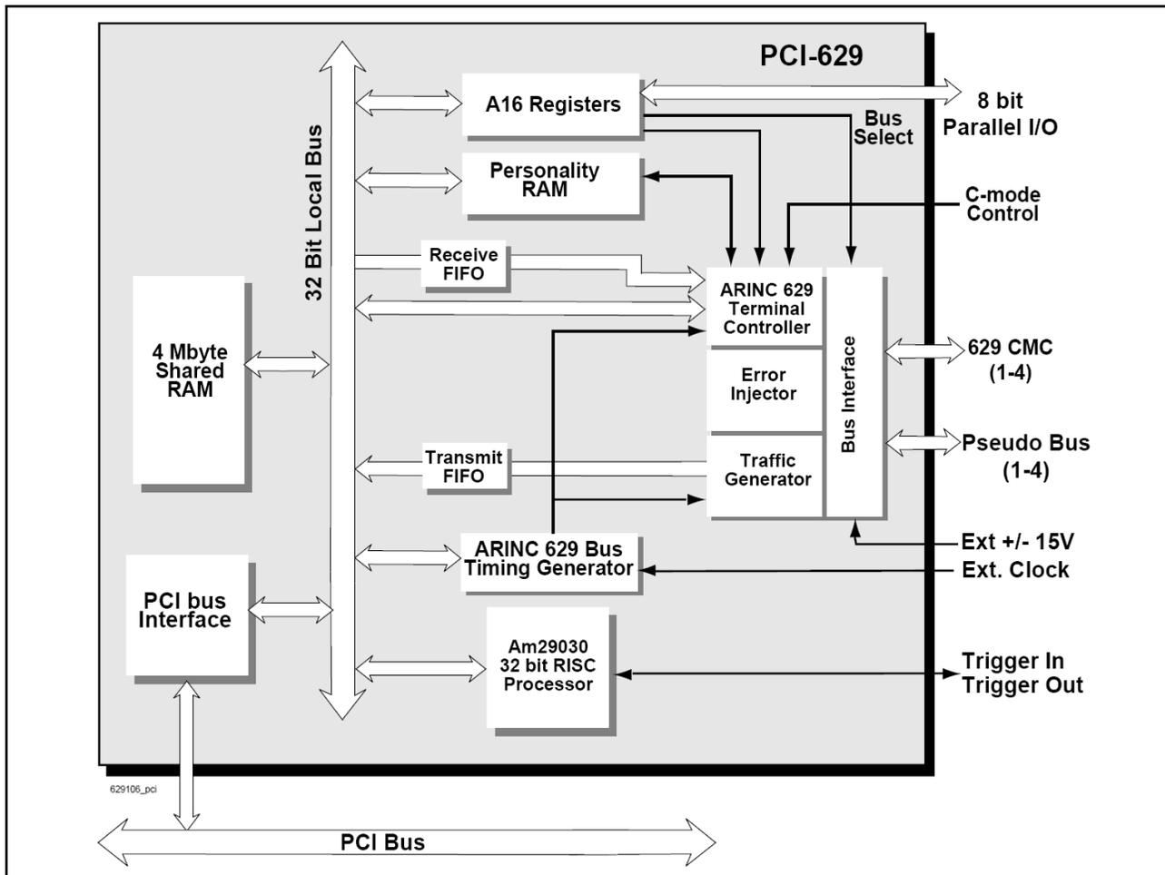
Figure 1. Block Diagram
