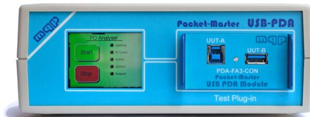
*The Packet-Master USB-PDA from MQP is the world's first dedicated Power Delivery Analyser.*
